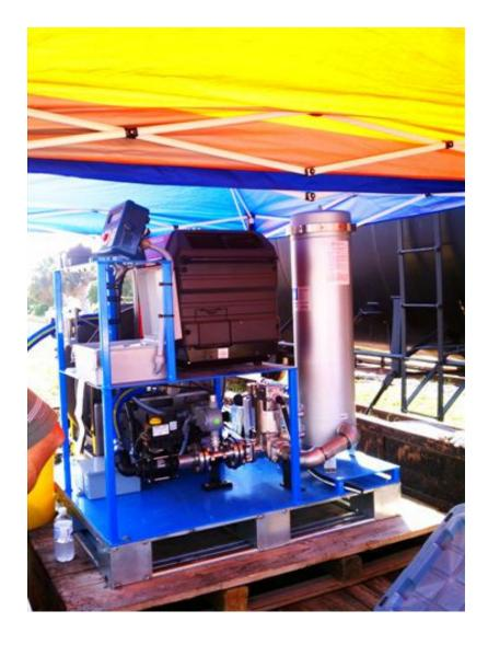
DEF stainless steel pump, SS filter housing with 7 individual DEF 1 micron filters inside.
